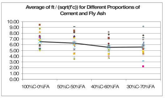
Figure 4: Variation of the ratio of tension and square root of compression strength with the fly ash content
