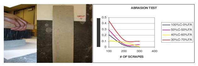
Figure 5: Scrapping test performed to a concrete plate to simulate the abrasion effect on concrete with different proportion of fly ash.
