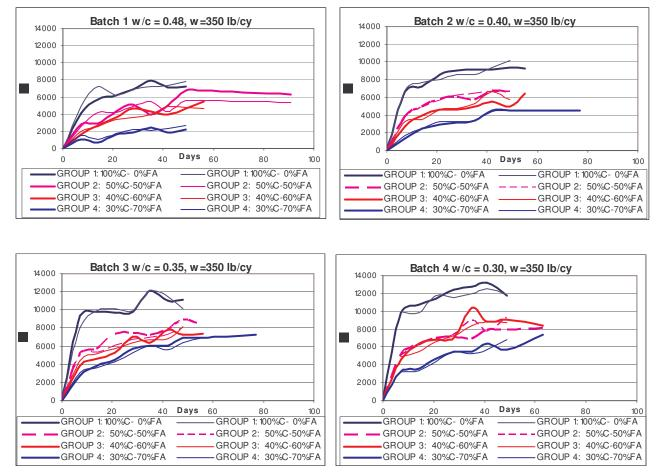
Figure 1: Compression strength versus time for concretes with different w/c ratio and a water content of 350 lb/cy.
