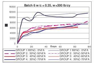
Figure 2: Compression strength versus time for concretes with different w/c ratio and a water content of 300 lb/cy.
